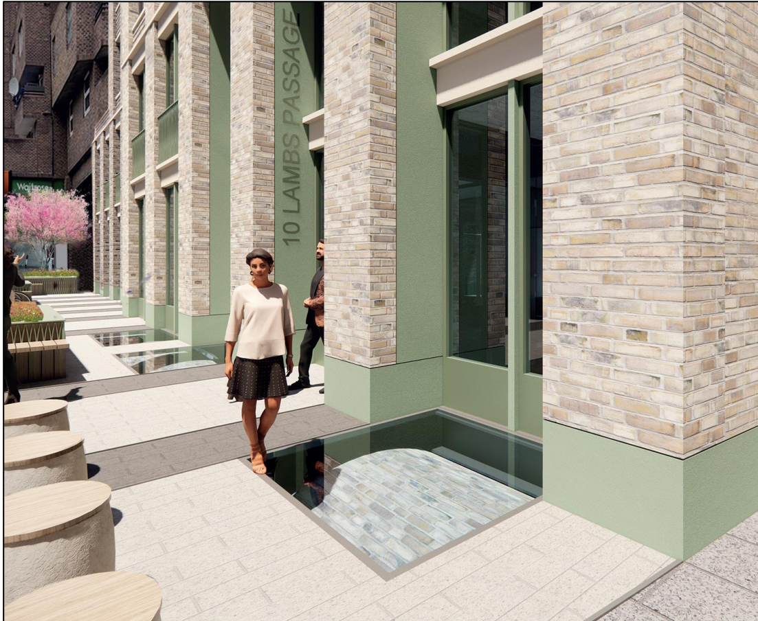
Figure 20: Indicative CGI outlining glazing to ground floor surface within the public realm to reveal the brickwork of the listed vaults below.
